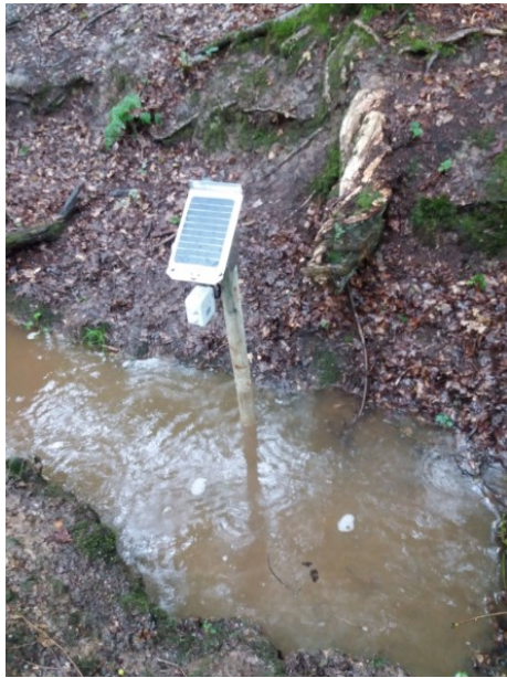
Figure 14 Water level sensor in stream channel and stream profile for Salmon's brook catchment, London
