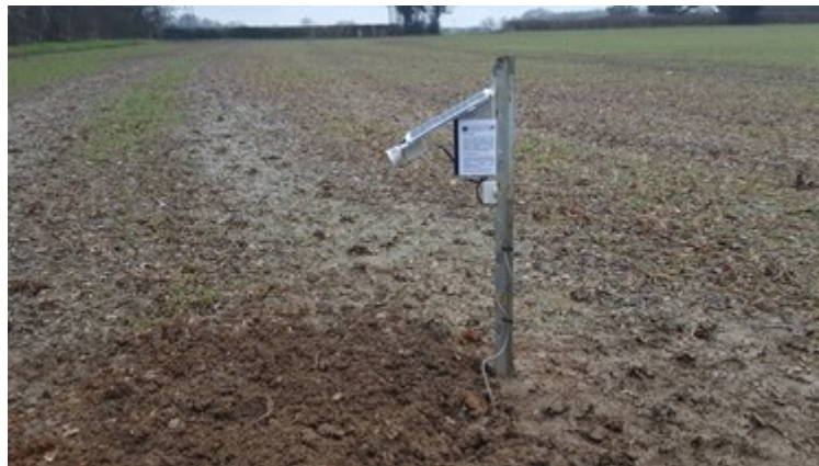
Figure 26 Soil moisture monitoring station installed on non-CA field in Hertfordshire
