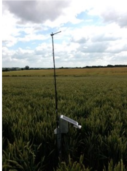
Figure 29 Soil moisture monitoring station installed on CA field in Suffolk
